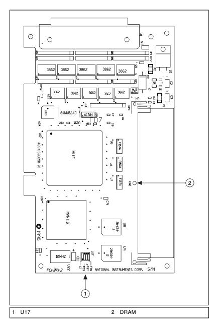
Figure 2-1. PCI-MXI-2 Parts Locator Diagram
